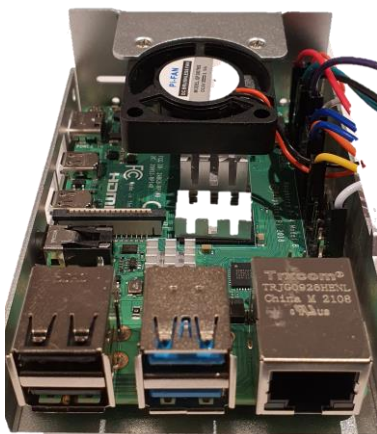
Figure 3.3 The Raspberry pi 4 model B is the core computer of the AOI
